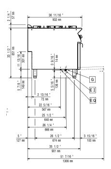
Electrical inlet (power) Gas connection
